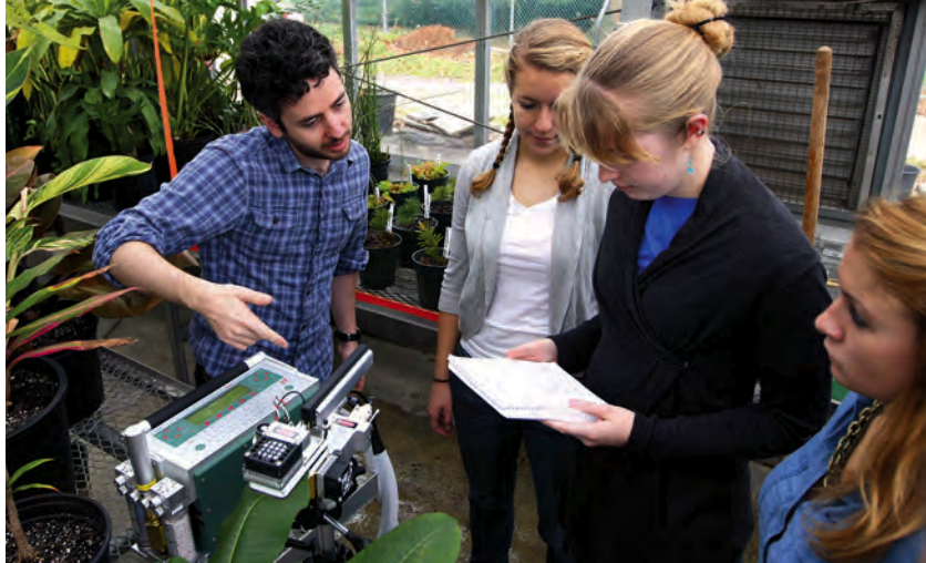
Assistant Professor of Biology Jonathan Wilson shows biology majors (left to right) Anna Rayne, Kelsey Capron and Emily Dutrow (all '12) how to measure rates of photosynthesis using the new infrared gas analyzer.
