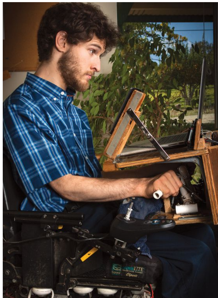
Carl Sigmond '13 worked with several collaborators on campus to refine a DEVICE HE INVENTED that attaches to his wheelchair and allows him to type using two levers.
