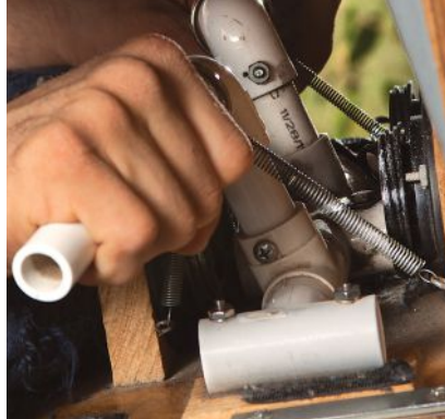
Sigmond moves the two levers on his LEVERBOARD forward and backward in different sequences to input text and control his computer.
